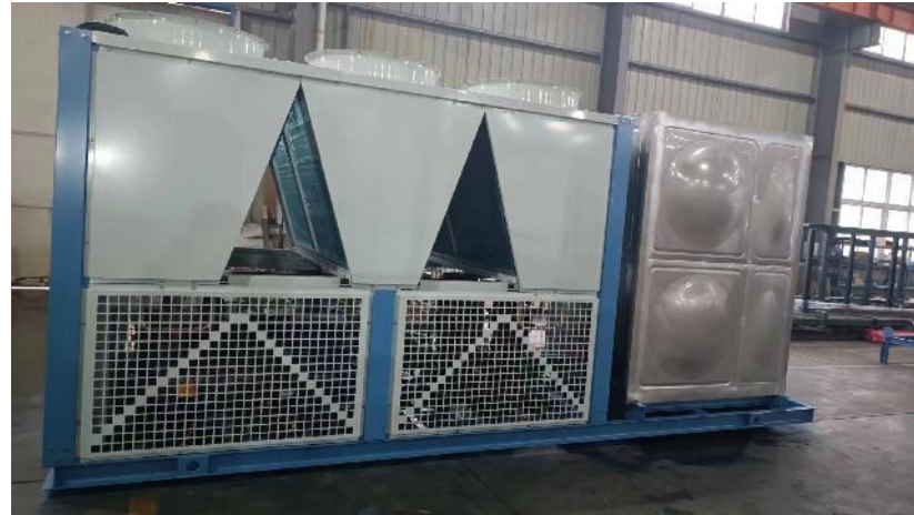
Air cooled Scroll Chiller/Bitzer&Copeland
