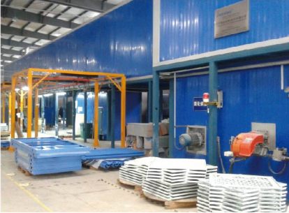
静电粉末喷涂生产线 Static electricity powder painting production line
